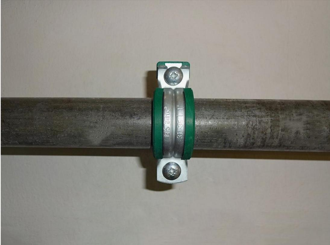
Fig. 2: Meas. 4: Bifix® G2 with insert, 4" (108 - 115 mm), connection M8/10, with EPDM-rubber (23 x 4,20 mm)
